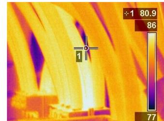
Over heated power cable to a circuit breaker.
