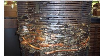
Catastrophic transformer failure in an industrial plant.
