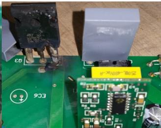
Gate driver network is susceptible to low-level voltage transients.
