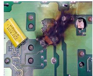
Failure on medical-grade power supply caused by voltage transient occurring in an Intensive Care Unit (ICU)
