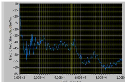
Radiated emissions (2 to 150 kHz) from a solar PV farm at 2:30 pm one clear sky afternoon.
